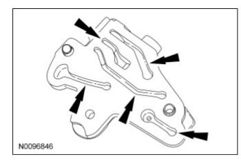
3. Inspect the <u>VCT</u>housing for pitting, cracks or damaged sealing surfaces. Install a new <u>VCT</u>housing if damaged.
