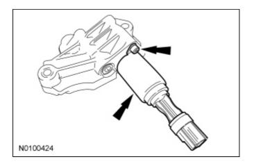
2. Clean the mating surfaces and oil passages with metal surface prep. Follow the directions on the packaging.
